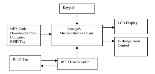
Figure 1: Block Diagram of RFID/Password Door Access Control System.
