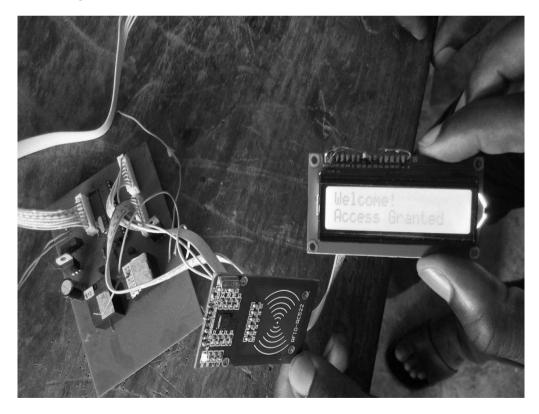
Figure 3: Components of the access control system on workbench.
