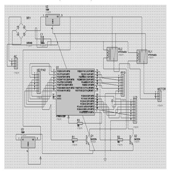
Figure 2: RFID/Password door access control system circuit diagram using PROTEUS
